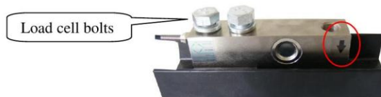
Photo 12 – Load cell connected to base unit
