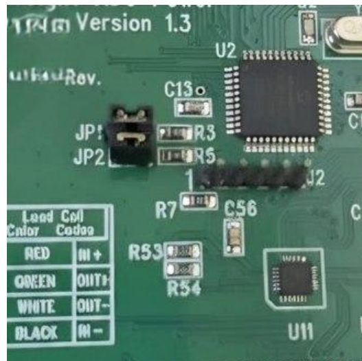
Photo 2: Jumpers in the Silo A/D card
