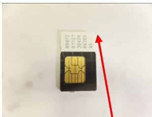
Photo 1 - SIM card Diagonally cut corner
