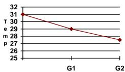
To Enter temperature reduction of 2°C in 7 days, press on 7 and than on 2 than on 0 and than on enter. On the display will appear: 7 2.0 G1 Press on data key, next group will appear.
