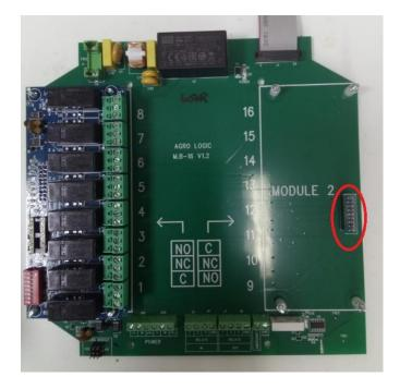
In the above picture, only 1 relay module is installed on the ver 1.2 relay board. The 1 empty module slot have the relay plug installed.
